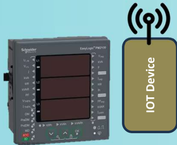
Power Meter at Machine
